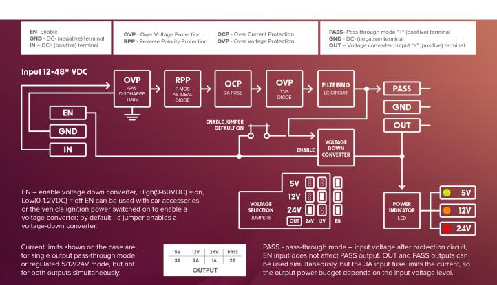
to be used in 12, 24 and 48 VDC automotive/vehicle electric systems, absolute maximum voltage ininput +60VDC, min input 9VDC
