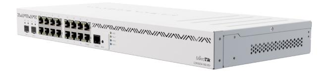
The new router has 18 wired ports, including 16x Gigabit Ethernet ports and two 10G SFP+ cages. It also has a RJ-45 console port on the front panel.
