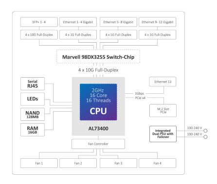
Each group of 4 ports has a separate full-duplex connection to the switch chip. No bottlenecks here. You can expect switch-like throughput in most setups.
