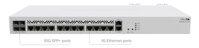
Obviously, you need the right connectivity to harness this power. There are **four 10G SFP+ ports.** They have a separate, full-duplex line connected to the Marvell Aldrin family switch chip. Then we have Gigabit Ethernet ports. 12 of them are running through the Marvel chip. And there is another Gigabit port connected directly to the CPU. For management purposes.
