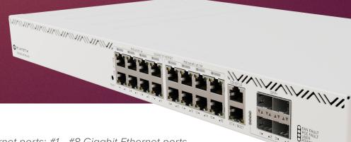
There are 17 Gigabit Ethernet ports: #1 - #8 Gigabit Ethernet ports with 802.3af/at PoE-out, #9 - #16 802.3bt PoE++ ports, and an extra Gigabit Ethernet port for management purposes. There's also a console port, and four 10G SFP+ fiber ports for uplink.
