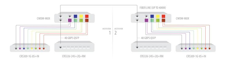
You can use a single optical fiber cable to create up to eight independent 1.25Gbps SFP (up to 40km) or 10Gbps SFP+ (up to 10km) links - saving plenty of time on money on installation or leasing of additional fibers. You can even use 1.25Gbps modules and 10Gbps modules at the same time. CWDM MUX/DEMUX modules are passive devices and there is no power source required.
