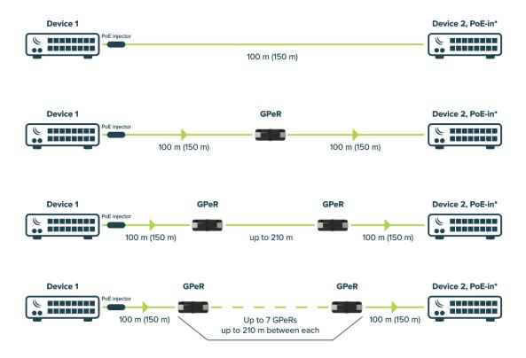
\* Voltage drop on the cable and on GPeR units needs to be taken into account when calculating PoE-in possibility, in case of insufficient power take off PoE jumpers to disable Passive PoE passtrough and use other power source for Device 2.
