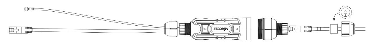
3. Follow the diagram sequence for inserting your ethernet cable. Lastly screw the Small Caps on both ends onto the Outdoor case tightly.
