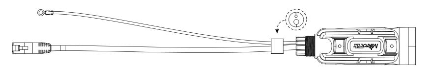
2. Take the rubber plug and fit it onto the cables. The cables must be placed in the matching hole size of the rubber plug.
