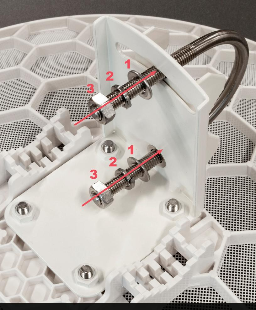
Use the provided M8 washers and nuts in the order that is specified in the image. Tighten the nuts with the 1/2 wrench.
