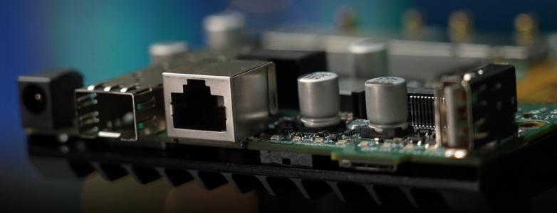
This modular board features a modern Qualcomm Maple CPU based on the ARM architecture, a USB port for extra storage or other needs, **Gigabit Ethernet with passive PoE-in, 2.5 Gigabit SFP** for fiber connectivity, and a **free miniPCle slot** that allows further customization. You could, for example, add an LTE modem for a mobile internet backup – we've added a NanoSIM slot on the bottom! But there are other options, like adding a gateway for LoRa IoT setups, such as our R11e-LR8!
