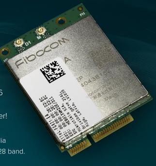
Carrier aggregation allows the R11 to use multiple bands simultaneously. That is a huge advantage in areas with many LTE users. It provides better responsiveness in a crowded environment and higher efficiency for weaker signal situations in the countryside. Depending on the service provider, we have seen Internet speed doubling in rural areas after switching to carrier aggregation!
