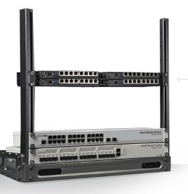
Compatible with all MikroTik (and other vendor!) devices that would fit in a standard 19" rack. But there's more! With the small K-79 accessory kit, you can fit up to four RB5009UG+S+IN routers in a single 1U rackmount space or up to 40 routers in total!
