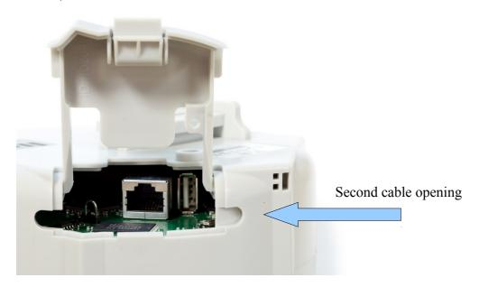
If you would want to mount the SXT horizontally, you need to use the second cable opening, so that the Ethernet cable goes straight down from that position. By default this opening is not accessible, you need to use a drill or a sharp knife to open the second cable opening. The second cable opening could also be used for grounding wire or USB cable.
