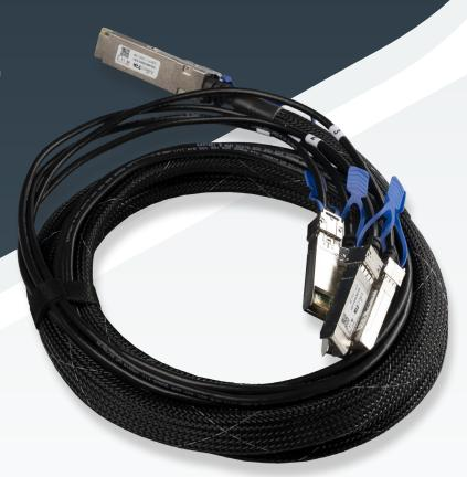
XQ+BC0003-XS+ is a QSFP28 to 4x SFP28 break-out cable. This addition to the MikroTik 100 Gigabit product line allows you to connect multiple 25 Gigabit devices to your CRS504 or CCR2216. With the integrated SFP28 modules, connecting numerous devices becomes as simple as it gets. The cable is 3 meters long – the perfect length to reach all the necessary spots while keeping your server room neat and tidy.
