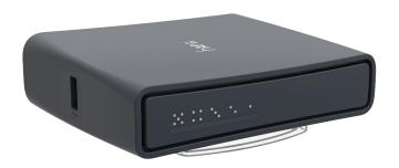
The hAP ac lite can be powered from the power jack or with passive PoE from a PoE injector. The power adapter is included. Unit provides PoE output function for port 5 - it can power other PoE capable devices with the same voltage as applied to the unit. Maximum load on the port is 500 mA.
