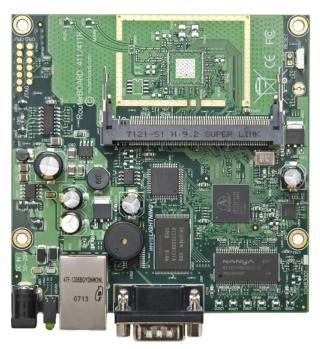
indicate that it can reach up to 3 times more throughput. This is the first of RouterBOARD products to use the new Atheros AR7100 CPU, and will require new RouterOS package files (mipsbe, see article on the left).
