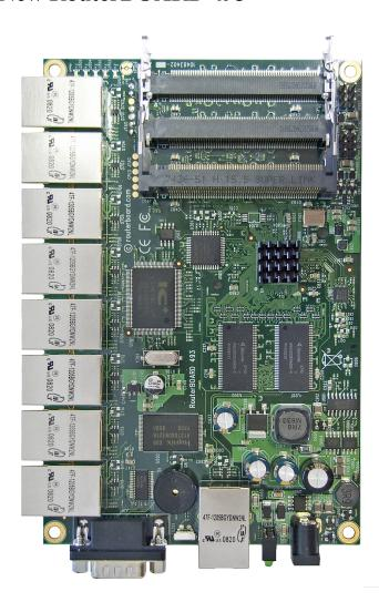
The much anticipated RB493 is here, replacing the successful multi port device RB192. Now all the ports are supported by the same powerful CPU as in RB411 and RB433. The new model also adds one more miniPCI slot.
