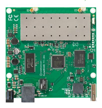
The RB711UA-2HnD is a small 2GHz wireless router, it has built in wireless with **two chains**, a USB port and PoE/Jack powering support. **Output power up to 1W!!!**
